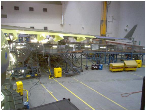
Two Clayton Vacuum Systems attached to wing stands, and one to the tail stand
