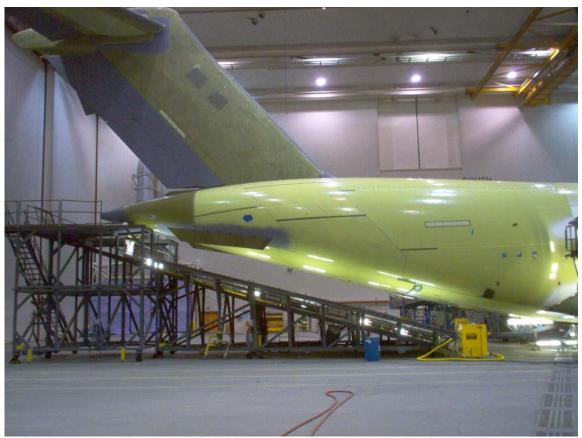
Clayton DustMaster Cyclones Attached to tail ramp
