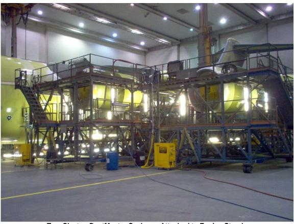
Two Clayton DustMaster Cyclones Attached to Engine Stands
